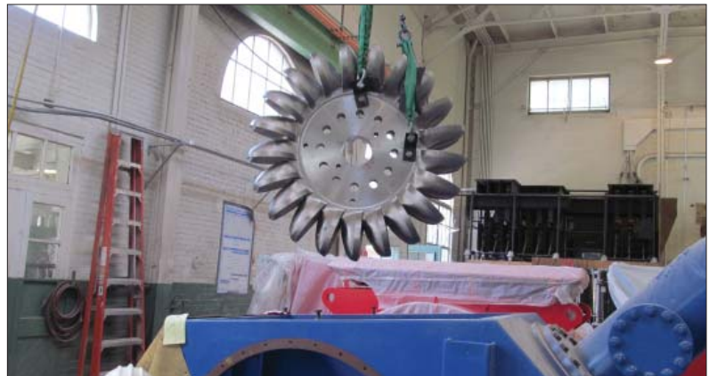
Opposite, the water that rages down Allison Creek will soon be used for additional hydropower Top, long-leadtime equipment similar to what was purchased for the Allison Creek Hydroelectric Project Above, a Pelton Wheel similar to what will be used for the project
